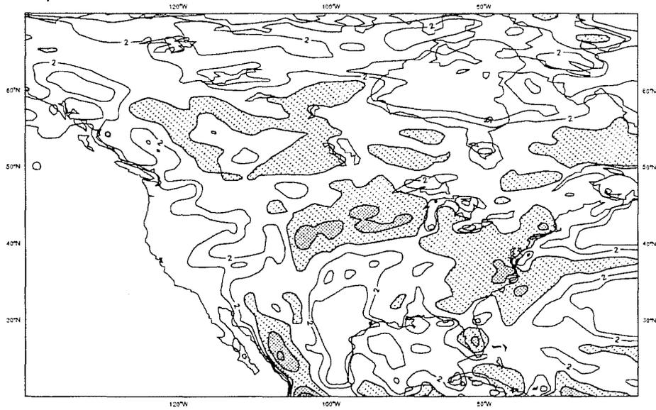
Fig 5 30-day average precipitation (mm/day) from ECMWF Cycle 48 T-106 forecast from July 1, 1993, using wet July 1 soil moisture, corresponding to unstressed evaporation. Contours are at 1, 2, 4, 8 mm/day.
