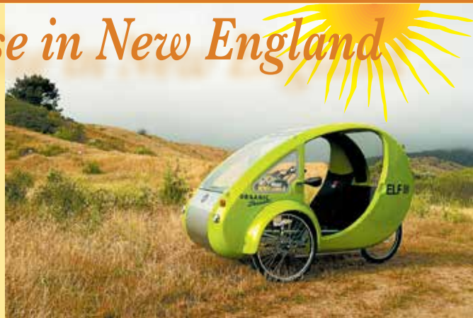
Electric-assist tricycle with solar panel on roof. Photo courtesy of Organic Transit.
