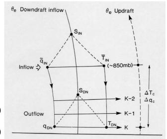
where  $\overline{T}_{IN}$ ,  $\overline{q}_{IN}$  are the grid mean values at the downdraft inflow level, and  $\Delta T_c$ ,  $\Delta q_c$  are the changes of T,q along the downdraft descent path (defined positive).
