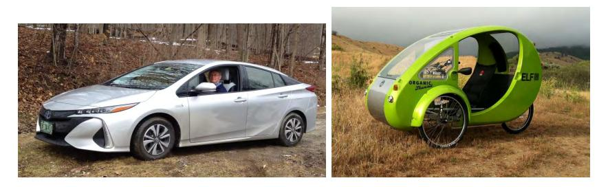
>3000lbs and 135 mpg Payload: 750 lbs at 65 mph 180lbs gets "1800 mpg" or 100 mp(1000Cals) Payload: 350lbs at 25mph
